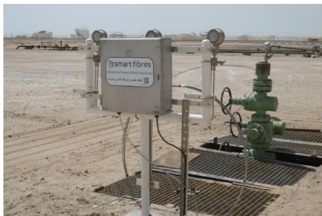
A DPTS Instrumented Oil Well, Oman
